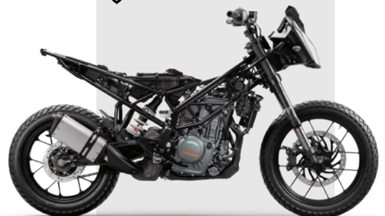
Lightweight & Stable Trellis Frame Inspired By KTM 450 Rally
